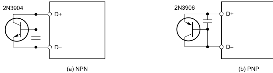
Figure 7-6. Remote Temperature Sensor Using Transistor
