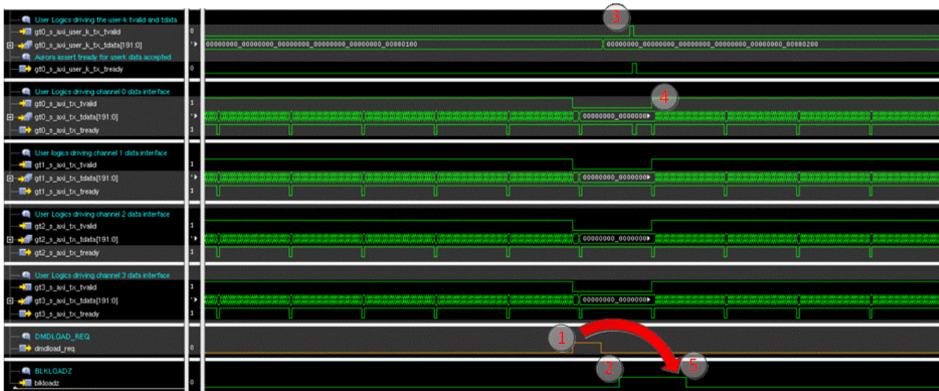
Figure 7-5. End of Block DMDLOAD_REQ Assertion Followed by New Block Control Word Waveform
