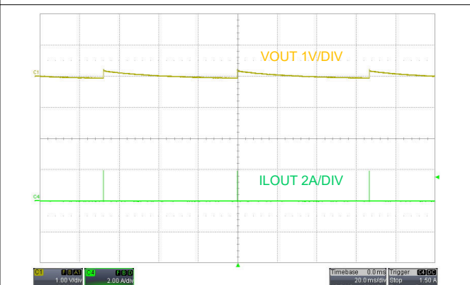
Figure 7-10. No Load Operation in PFM Mode, V_{SUPPLY} = 48V , I_{LOAD} = 0A
